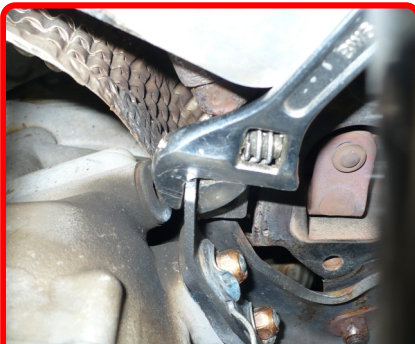
Step 4: Check for proper alignment of the bracket to the lever. The lever is to be centered with the threaded nut. Adjustment may be necessary by using a small wrench or vice-grips to bend the tab.
