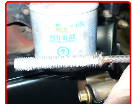
Step 7: Apply Anti-Seize to threads of each end of the Lock Cable.
