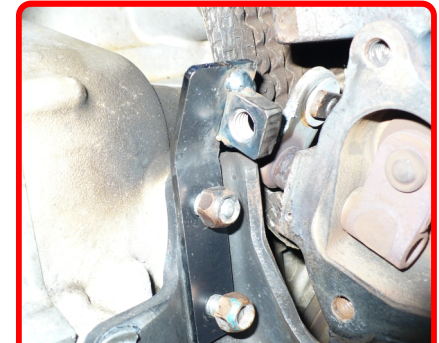
Step 3: Install Inner Bracket using the factory lock retainer & lock nuts.
