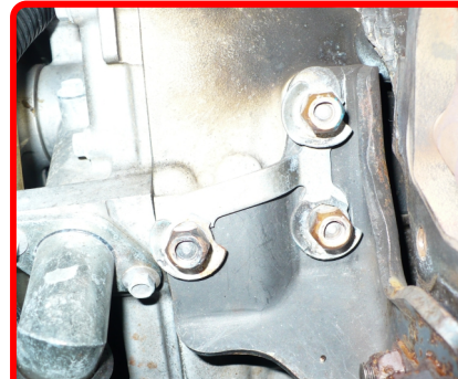
Step 2: Remove the 3 locknuts from the Turbo Support Bracket.
