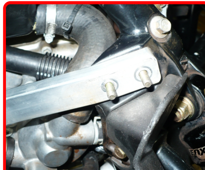
Step 5: Remove the 2 nuts on the Muffler Support Spar.
