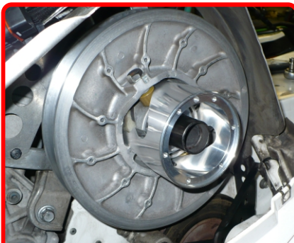
Step 9: Install the clutch on the sled.
