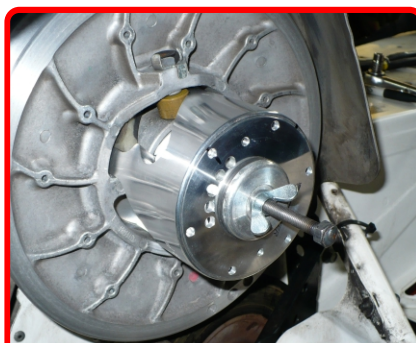
Step 14: Tighten wingnut until the outer cover meets the helix.
