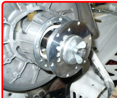
Step 11: Using the installer tool/bolt with existing sheave adjuster install the new spring in the center hole of outer cover. Screw tool/bolt into the jack shaft approximately \frac{1}{4} to \frac{1}{2} inches.
