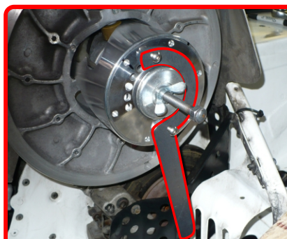
Step 15: Using 2 of the supplied cover bolts, install handle onto the cover.
