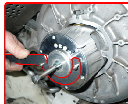
Step 16: Twist clockwise until the marked holes line up (roughly 70 degrees). With Blue Loctite, install the two (2) cover bolts and tighten.
