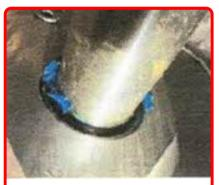
**Step 7: IMPORTANT** - Initial greasing is 20-25 shots from a hand held grease gun. Regrease with one shot every 500-1000 miles.
