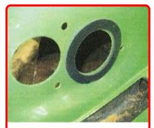
**Step 4:** On the tunnel area behind the caliper, clean and install the supplied *Rubber Seal*. **NOTE:** If kit is installed in a new sled, a new caliper bearing is not required. If a used sled, it is recommended to replace the caliper at this time.
