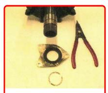
**Step 2:** With track shaft removed from sled, remove the *snap ring, inner seal and the bracket*. Discard the inner seal and the bracket.
