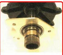
**Step 3:** Make sure the bearing area is cleaned and free of debris. Install the Bearing Bracket Update Kit onto the shaft & reinstall the snap ring.
