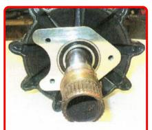
**Step 5:** Apply a small amount of grease to the inner & outer shaft service. Place the shaft back in the chassis with the bearing bracket in this position.
