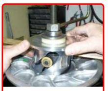
**Step 12:** Apply a small amount of spring pressure while rotating helix clockwise by hand. Once the helix starts over the humps, screw down the spring pressure until helix starts to rotate down into the sheave.
