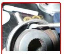
**Step 7:** The holes in the hub should be chamfered on the inside where it contacts the edge of the hole. This can be done by using a die grinder or Dremel tool.
