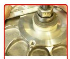
**Step 16:** Using supplied lever tool, apply enough clockwise pressure to align the helix holes. Use Blue Loctite to install the 2 bolts, holding pressure on the lever. *It's easier with 2 people*. Install remaining 2 bolts & torque to MFG specs.
