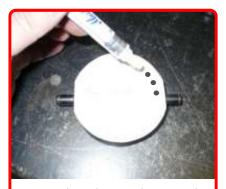
**Step 5:** Place the template over the hub & mark the three (3) holes.
