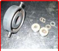
**Step 3:** Remove the rollers from the stock hub to avoid any damage while drilling the hub assembly.
