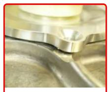
**Step 15:** Apply spring pressure until helix is about 1/16" from the sheave.
