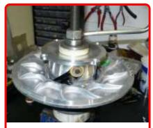
**Step 14:** Once sticks are removed continue applying pressure to the spring. Helix will rotate as spring pressure is applied.
