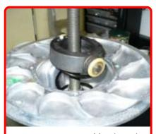
**Step 10: To Reassemble** place the sheave on the threaded rod along with the spring & hub assembly. Place the spring in the drilled hole in the bottom of the sheave.
