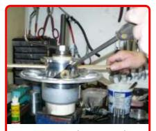
**Step 13:** Using a long screw driver, insert between the hub assembly & helix, applying a small amount of pressure so stick can be removed. *Repeat for opposite side.*
