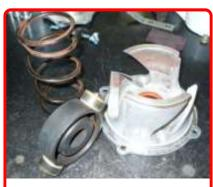
**Step 2:** Remove stock helix, spring and roller hub.
