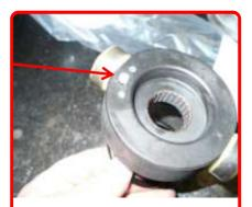
**Step 9:** Reassemble rollers, washers & circlips back on the hub assembly. Using the supplied spring, place the white tipped end in the middle hole of the hub assembly.
