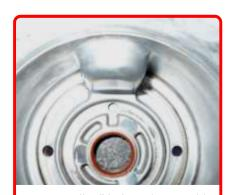
**Step 8:** Drill ¼" hole in the movable sheave spring pocket (as indicated).
