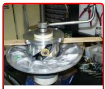
**Step 11:** Start helix onto the rollers and now insert the two (2) pieces of the supplied stick to support the hub while spring tension is applied.
