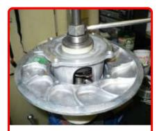
**Step 1:** Disassemble clutch using a piece of threaded rod or clamping device.
