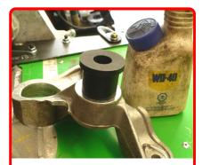
**Step 12:** Install the urethane mount (without the insert) into the factory engine mount first. Use a little WD40 to help with this installation.
