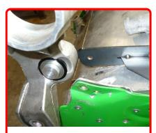
**Step 13:** Install the insert into the urethane.
