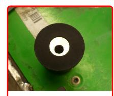
**Step 16:** Recheck the alignment. If more adjustment is required, use the larger offset insert.
