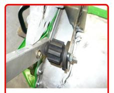
**Step 5:** Lightly tighten as to align bracket to the mount for proper fit before drilling the two holes for the aluminum support brackets (underside of tunnel).
