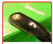
**Step 3:** Remove both running board support bolts (right & left). Place the corresponding supplied bracket (left for clutch side/right for chain case side) under running board support hoop and reinstall bolt.
