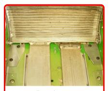
**Step 7:** Drill out the two remaining holes in the support brackets. Install supplied aluminum support brackets on the underside of the tunnel using the supplied nuts and bolts (use LocTite on all fasteners).
