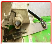
**Step 4:** Using either the supplied urethane mounts or factory rubber mounts, install using the factory bolts.
