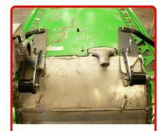
**Step 8:** Tighten the running board support bolts and aluminum bracket bolts. Remove mocked-up urethane or rubber mounts (to be installed in the factory engine mounts).
