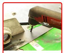
**Step 6:** Using a 5/16 "drill bit (use of a right-angle drill is preferred)
