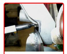
**Step 9:** Prior to installing factory right side/chain case side alumin. engine mount, it is recommended to trim the area as pictured to facilitate clearance on the new bracket.
